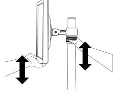
**5.2** Lift/Lower Screen to the desired height. Move both Screen and Micro Head assembly together.
