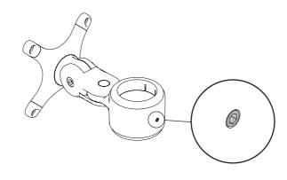
2.2 If the Grub Screw is removed the Micro Head will be free to rotate 360degrees about the pole
