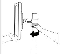
**5.1** Unlock Handgrip ensuring both screen and Micro Head are supported.
