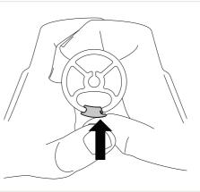
**B.** Press down firmly onto the other edge of the Cable Stop and hold. This allows the rear profile to flex in place.
