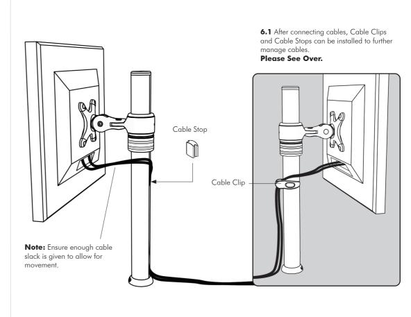
**Note:** If Focus Micro is to be used in a multi user environment, use the supplied Cable Clip to secure the display's cables to the Pole.
