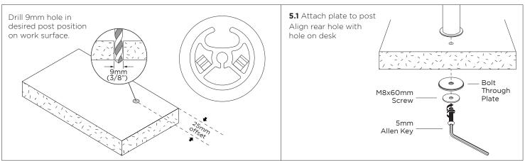
5. Installing bolt through
