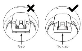
**5.3** Push the lever down to secure monitor to the arm assembly
