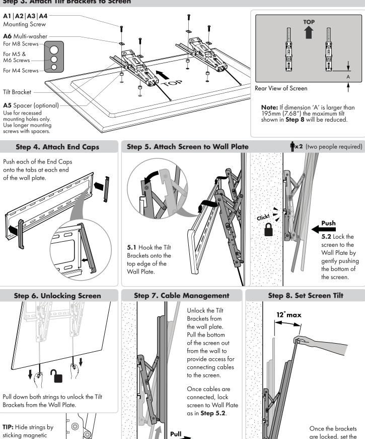
sticking magnetic pendants onto the Tilt Brackets behind the screen.
