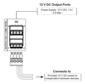
When the total current exceeds the maximum threshold, the DC power overload LED lights orange, and the alarm beeps for 3 seconds, while turning the channel(s) off.
