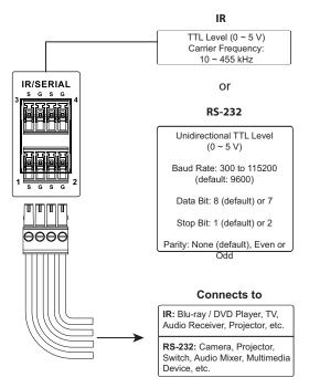
Connect to IR and/or RS-232 devices. By default, these channels are set to transmit IR signals.
