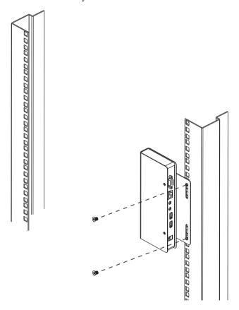
**Note:** These screws are not provided. We recommend that you use M5 x 12 Phillips Type I cross, recessed type screws.
