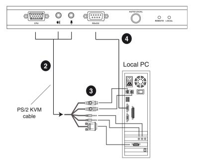
**Note:** The serial port on the CE350L / CE370L connects to the computer; the serial port on the CE350R / CE370RQ (not shown) connects to a serial device (optional).
