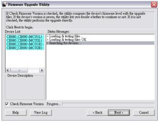
The Utility inspects your installation. The Local and Remote Units are listed in the **Device List** panel and automatically selected for upgrade.
