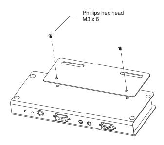
2. Screw the bracket into any convenient location on the rack.
