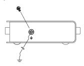
2. Make sure that the computer that the CE750AL connects to and the monitor that the CE750AR connects to are properly grounded.
