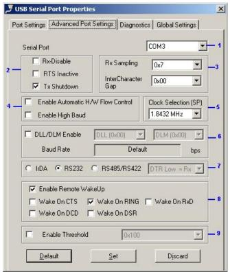
On this tab you will find many configuration settings which can be customized according to your requirements. Click **Default** to reset all values their original setting, **Set** to apply changes, or **Discard** to remove changes before they are applied. This tab has 9 sections, described in the table below:
