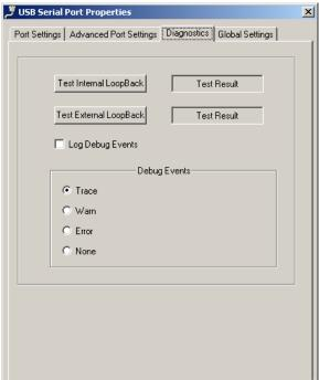
This tab is used to conduct Internal and External Loop-back diagnostics. Click the **Test Internal LoopBack**, or **Test External LoopBack** button to begin a test and view the *Test Result*
