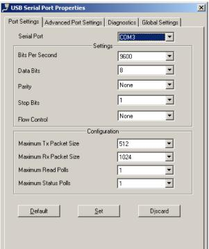
There are two sections on the *Port Settings* Tab: *Serial Port section* and *Configuration*. Click **Default** to reset all values their original setting, **Set** to apply changes, or **Discard** to remove changes before they are applied.
