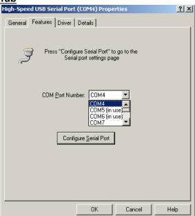
This tab is used to change the COM port number and configure the port. Use the *COM Port Number* drop down list to select the serial port you want to configure.
