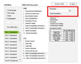
In the **Resolution** drop down menu, choose a resolution with values that fit the attached monitor/display device and click **Save**.
