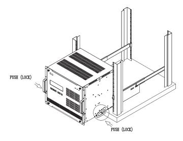
3. Screw the front panel to the rack.
