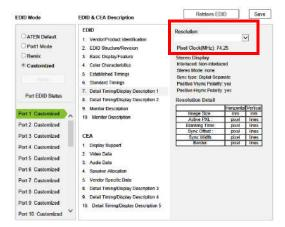
In the drop down menu, choose a resolution with values that fit the attached monitor/display device and click Save.
