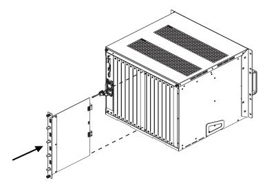
3. Slide an input board into a right side slot and then tighten the screws to secure the board to the VM3200.
