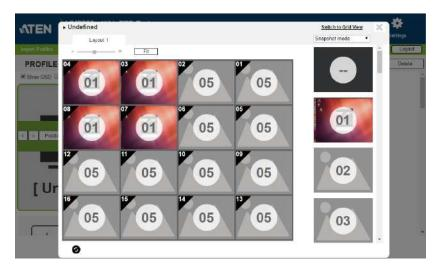
The *Change Input* page displays still image frames of output configuration, the left panel shows the profile's output configuration, and the right column lists the available inputs. The page provides the following options:
