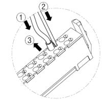
Push the wire connected with the crimp terminal towards direction 1 to complete the connection.
