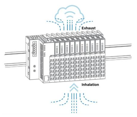
To minimize the interference and impact of products, wire, and peripheral devices, you must install the ARIO to meet installation distance.
