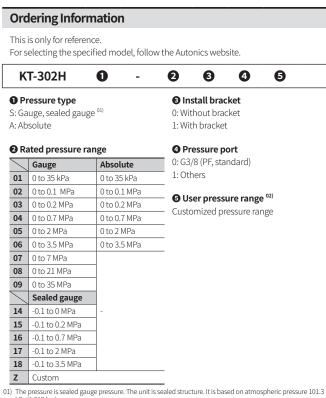
(k) The pressure range is set to customized pressure range. (select "Z" at (2) Rated pressure range)
