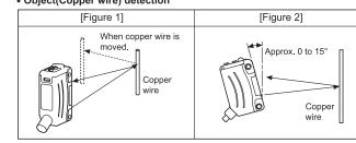
\*Mount sensor slanted at an angle ranged 0 to 15° shown above as [Figure 2] for stable detection to detect as shown in [Figure 1].
