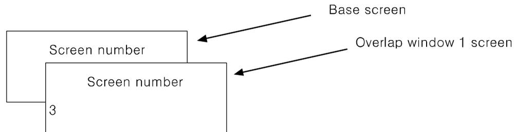
Overlap window 2 is not overlapped because the value of overlap window 2 device is not an existing base screen number.
