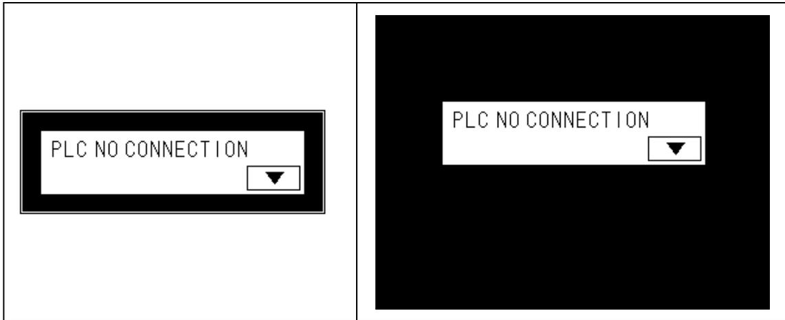
Touch 'CLOSE' and error message dialog box disappears. If connection error is not resolved after 5 seconds, error message appears again on the screen.
