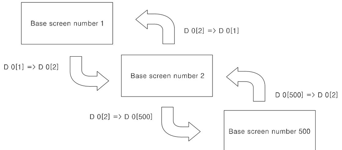
If there is no screen number corresponding the device value of screen data, error message appears.
