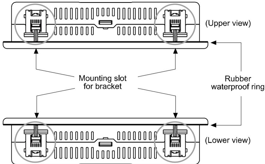
1st Set a rubber waterproof ring after placing the ring's joining part under the GP.
