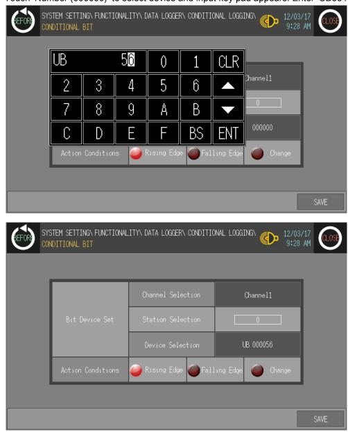
3rd Touch 'Number (000000)' to select device and input key pad appears. Enter 'UB56'.
