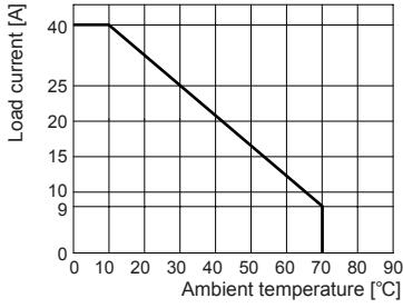
⚠ Since effectiveness of the heat radiation is decreased when multiple SSRs are installed closely, please supply less than 50% of the rated load current.
