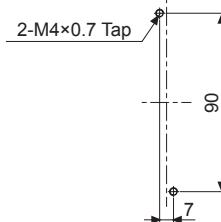
※ Screw tightening torque for mounting : 1.8 to 2.5N·m
