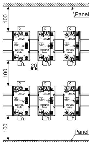
※ When installing multiple SSRs, please keep space between SSRs for heat radiation.
