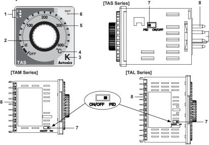
1. Deviation indicator: It shows deviation of present temperature (PV) based on set temperature (SV) by LED.
