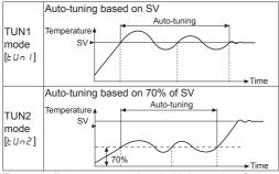
To manually stop auto-tuning, hold the AT key for 5 seconds. When auto-tuning is stopped, the controller maintains the PID value before auto-tuning. TZ Series supports 2 auto-tuning modes.
