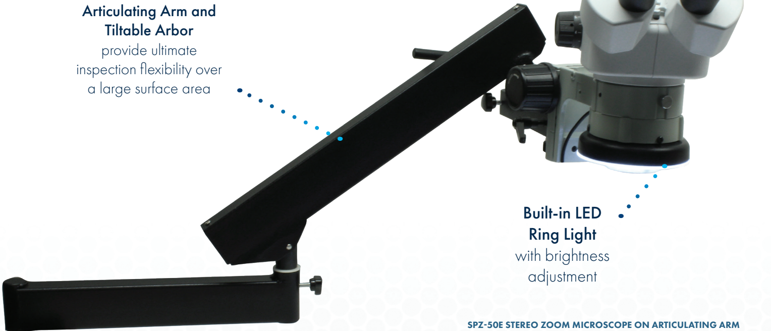
SPZ-50E STEREO ZOOM MICROSCOPE ON ARTICULATING ARM STAND WITH ARBOR AND FOCUS MOUNT + RING LIGHT
