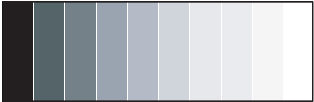
Figure 4-3. Typical Grey Bar Pattern for Adjusting Contrast
