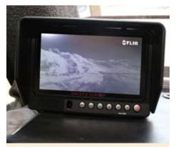
The thermal images produced by the PathFindlR are displayed on a 7" LCD display inside the trucks cabin. They help the driver to avoid accidents.
