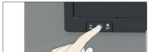
Fig. 17 Switch off appliance
