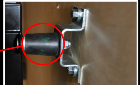
(4) Point Column Connection Dampening
