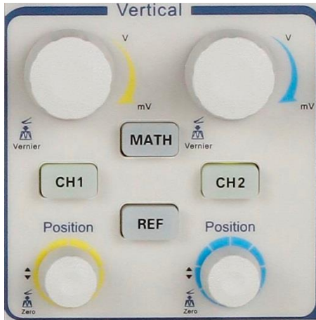
Figure 3.5 – Vertical System Controls
