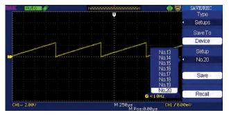
Minimize debug time by saving and recalling setups and waveforms from internal memory. Save and recall up to 20 different oscilloscope setups and 10 different waveforms.
