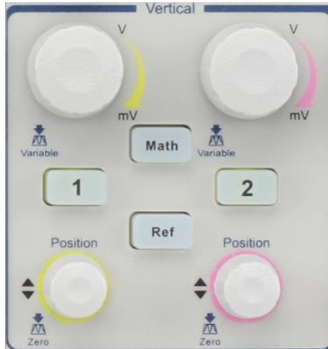
Figure 3.5 – Vertical System Controls
