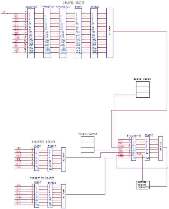
Figure 2 - Load Status Register Structure
