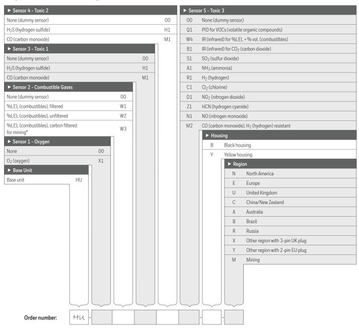
For example, the order number for a Honeywell BW™ Ultra configured for O<sub>2</sub>, %LEL (filtered), H<sub>2</sub>S, CO, and SO<sub>2</sub> and equipped with a black housing and North American power connectivity would be HU-X1W1H1M1S1-B-N.
