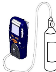
Figure 4.1 Bump Test / Gas calibration set up
