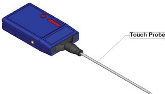
The patented Touch Probe accessory is a device that converts solid-borne sounds into airborne sound the Tru Pointe® Ultra can detect. For example, the sound of an internal leak in a water valve will travel to its surface. Touching the surface of the valve with the Touch Probe transfers the ultrasound into the probe and converts it to airborne ultrasound.
