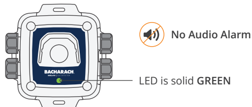
Figure 4-3 - Inspecting Connected MGS-410
