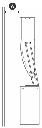
If this distance is not practical due to site conditions, maintain a distance of no less than 100 mm (4 in) and no more than 300 mm (12 in) between the top-front of the speaker and rear of the perforated screen, to avoid deterioration of audio performance.
