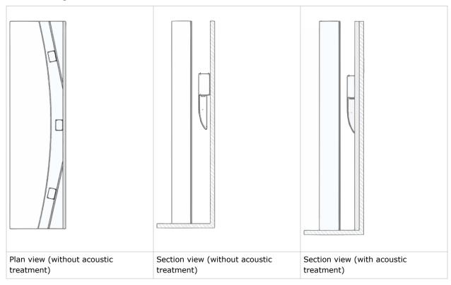
In the diagram, the speakers and subwoofers are connected using an L bracket, in a flown configuration. Alternatively, this configuration can be implemented with speakers and subwoofers connected using a tilt bracket and placed on a platform in front of the baffle wall.
