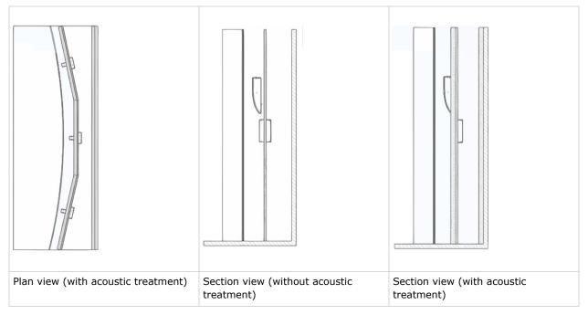
Acoustic treatment is required on both the front of the baffle wall and on the existing wall. Ensure that the front face of the subwoofers are flush with the front face of the acoustic treatment applied to the baffle wall.
