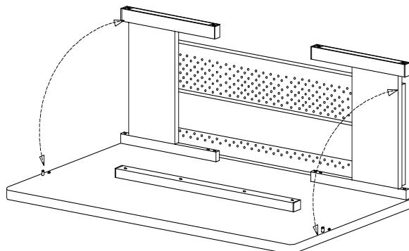
4.) Swivel the legs out and place them over the two locator posts that are attached to the bottom of the table top as shown in Illustration #3. Secure the leg to the table top using two Thumb Screws (C).
