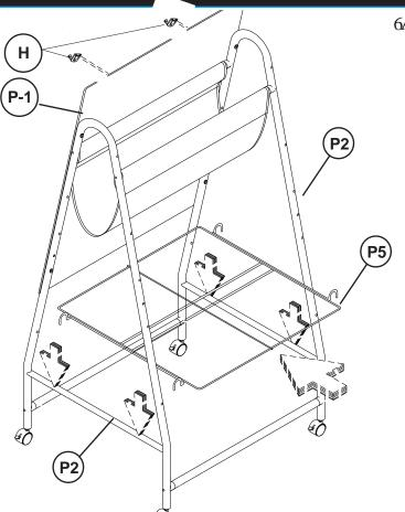
6A. Peel the paper off from the back of adhesive pad on Plastic Chart Support (H). Insert the 2 pins on the backside of the Chart Support (H) in the holes in the markerboard (P-1), as shown in Illustration # 6 and # 6-A. Firmly press the Plastic Chart Support
