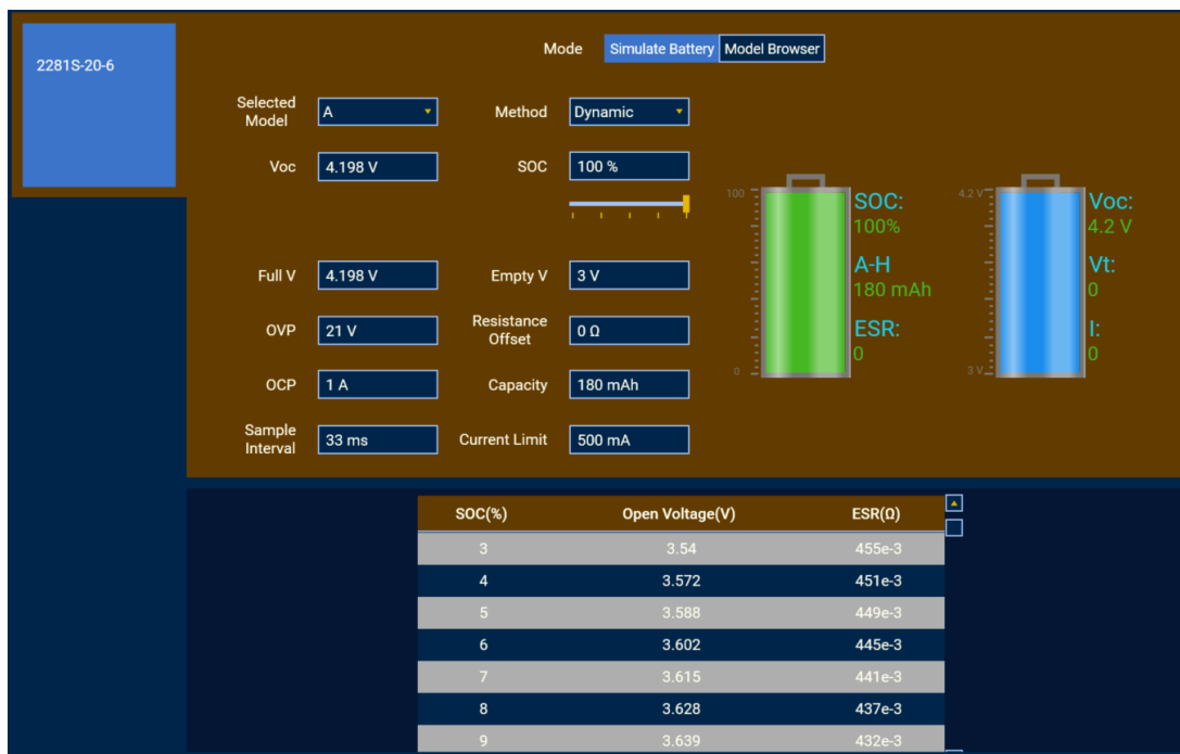
Figure 10: Simulate Battery in KickStart Software
