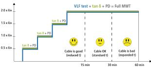
insulation. Moreover, a partial discharge measurement shows and locates the PD faults precisely. The highlight of MWT is the condition-based test duration: Provided it is permitted, the test duration can be shortened, which in turn lowers costs. This way, the cable is only exposed to the increased test voltage for the required duration.
