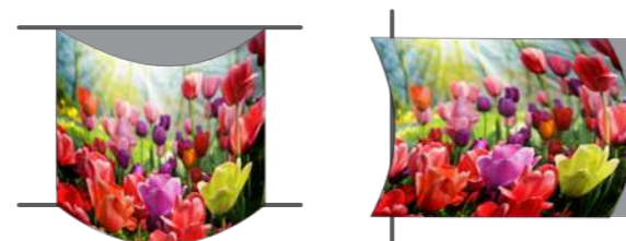
Surface Fit for Pincushion and Barrel
