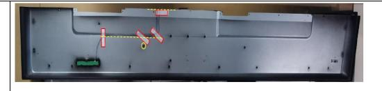
Remove the AC inlet ASSY and the key board & IR board.
