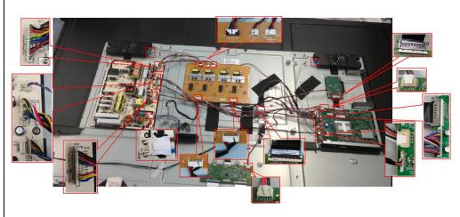
Remove the screws to remove the main board, power board, connector board and converter board. And then remove the Mylar.
