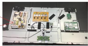
Take off the tapes and remove the IR board. Remove the speakers and the BKT\_OPS\_CHASSIS.
