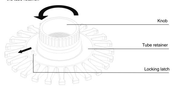
1.2 The tube holder may be filled in or out of the instrument. To remove, simply lift off the shaft. Place sample tubes into the tube holder and press down until seated. If less than 24 samples are used, they should be evenly distributed in the tube holder. If removed, the tube holder can then be replaced, making sure the two bumps on the holder line up with the indentations on the shaft.
