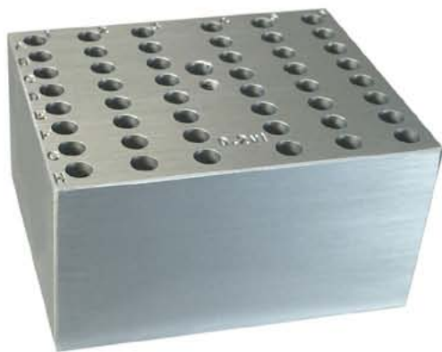
Catalog Number: BSW02 Capacity: 48 x 0.2 ml or 6 PCR tube strips Block Dimensions: 3.75 x 3 x 2 inches Hole Dimensions: 6.0 x 14.0 mm
