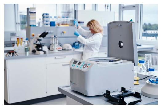
The Z287-A exceeds the limitations set forth by traditional microcentrifuges which are restricted solely to fixed angle rotors for microtubes. Instead, this compact, next generation model features an expansive line of swing out and fixed angle rotors options that accept microplates and test-tubes up to 50ml. We've designed this centrifuge to be our most compact and economical. A true workhorse for any lab requiring a centrifuge that can accommodate many fields of research.
