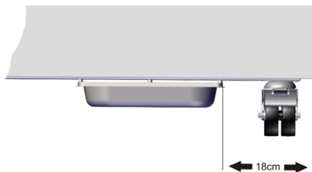
Figure 17: Positioning the condensate collection pan (front view)
