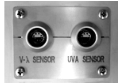
Figure 13: Lemo sockets to connect the light sensors
