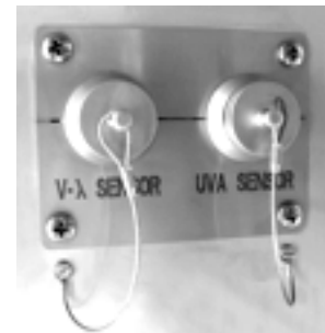
Figure 14: Connection sockets closed with protecting caps
