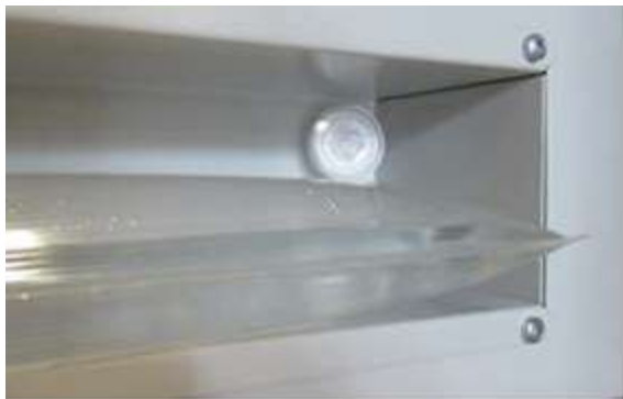
Figure 49: Location of the gas fine filter (sterile filter) in the recess for the freshwater bag
