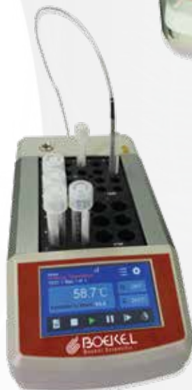
Two Block Unit with External Temperature Probe
