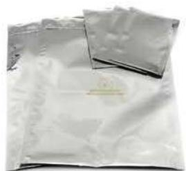
**Features:** Botron's antistatic shielding bags are metal-out and low tribocharging. Thus, ESD sensitive materials stored inside the bag will not generate a charge. The 3mil thick lining is puncture resistant and protects against corrosive materials. Comes with either zipper or flat applications. Provides rapid charge dissipation and 30% light transmission.
