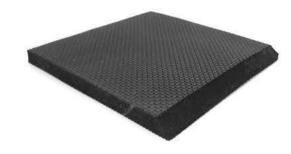
**Features:** Type EM Conductive Sponge rubber mats and runners designed to reduce strain from standing on hard surfaces. These slip and soil resistant mats are 5/8" thick with beveled edges on all sides. It exceeds both EOS/ESD and Department of Defense requirements. Available in black runners, and pre-cut floor mats with hardware.
