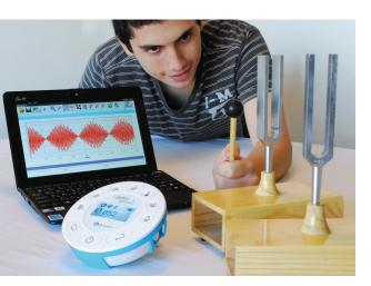
As a single multi-meter device, the Labdisc replaces all traditional meters and sensors in the lab. Yet, the Labdisc does not replace experiment materials and accessories such as glassware, chemicals, tuning forks, weights, etc.
