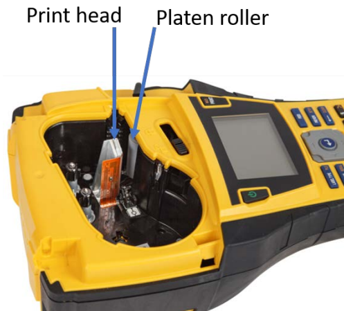
Figure 39 • Print head and platen roller in cartridge bay
