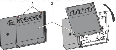
2. Loosen screws (1) and remove cover (2) towards the front.
